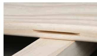
Local grooving, with a Lamello® type biscuit joiner or a router.
