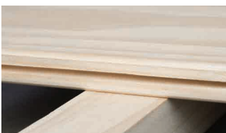
Grooving along the whole length, with a 4-sided planer or spindle moulder.
