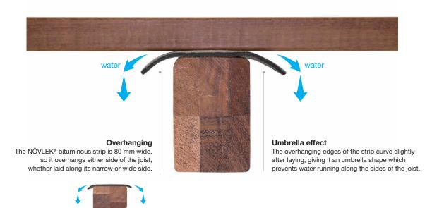
Joist laid on its wider side
